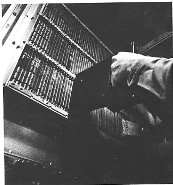
In-place card testing using hand-held test set.
