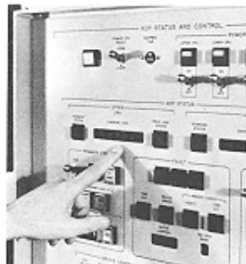
Readouts Indicate Faulty Area 1.0 min (Fig. C)
