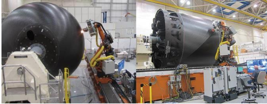
Figure 12: Carbon fibre is placed on the 5.5-meter cryotank using an automated tape placement laminator [ http://compositesmanufacturingmagazine.com/2014/10/composites-key-outer-space-applications-material/ ]
