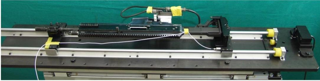
**Fig. 10** MSBS-5,56 K-01 during the recoil distance measurement.
