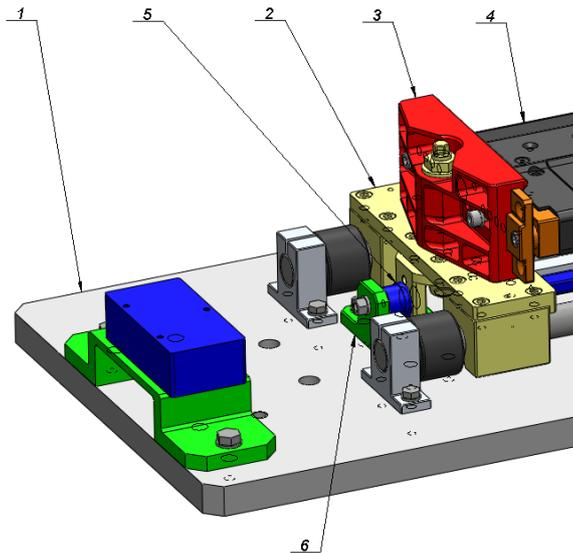
**Fig. 5** Test stand set for measuring the recoil force: 1 – base, 2 – rear cart, 3 – butt holder, 4 – examined weapon, 5 – force sensor, 6 – force sensor base.
