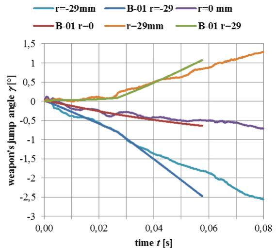
Fig. 18 Comparison of the B-01 rifle weapon's jump with the simulation results.
