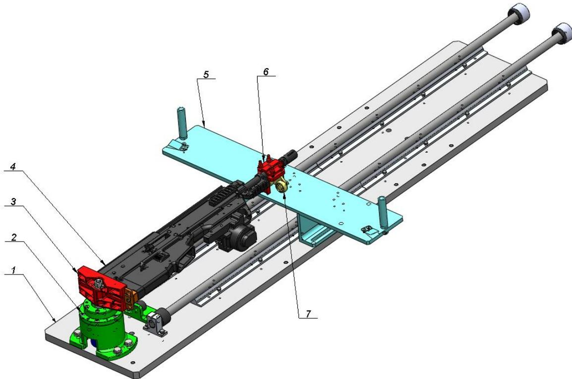
**Fig. 6** Test stand set for measuring the weapon's jump angle: 1 – base, 2 – turn axis base with the encoder, 3 – butt holder, 4 – tested weapon, 5 – table, 6 – barrel holder, 7 – transverse cart.
