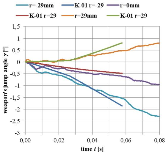
Fig. 17 Comparison of the K-01 rifle weapon's jump with the simulation results.
