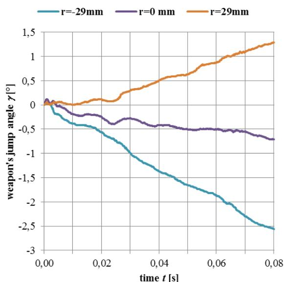
Fig. 15 MSBS-5,56 B-01 rifle experimental weapon's jump angle  $\gamma$  versus time  $t$ .
