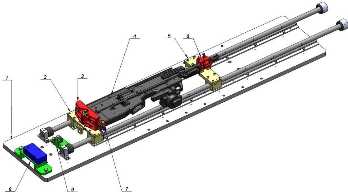
**Fig. 4** Test stand set for measuring the recoil distance and the weapon's acceleration: 1 – base, 2 – rear cart, 3 – butt holder, 4 – examined weapon, 5 – front cart, 6 – barrel holder, 7 – acceleration sensor, 8 – position sensor base with the sensor, 9 – force sensor base with the shock-absorber.
