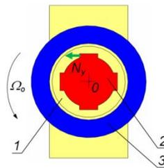
**Fig. 3** Physical model of the weapon's turn: 1 – the weapon, 2 – bullet, 3 – guides, 0 – barrel axis,  $N_y$  – force on the grooves,  $\Omega_0$  – weapon's turn angular velocity.
