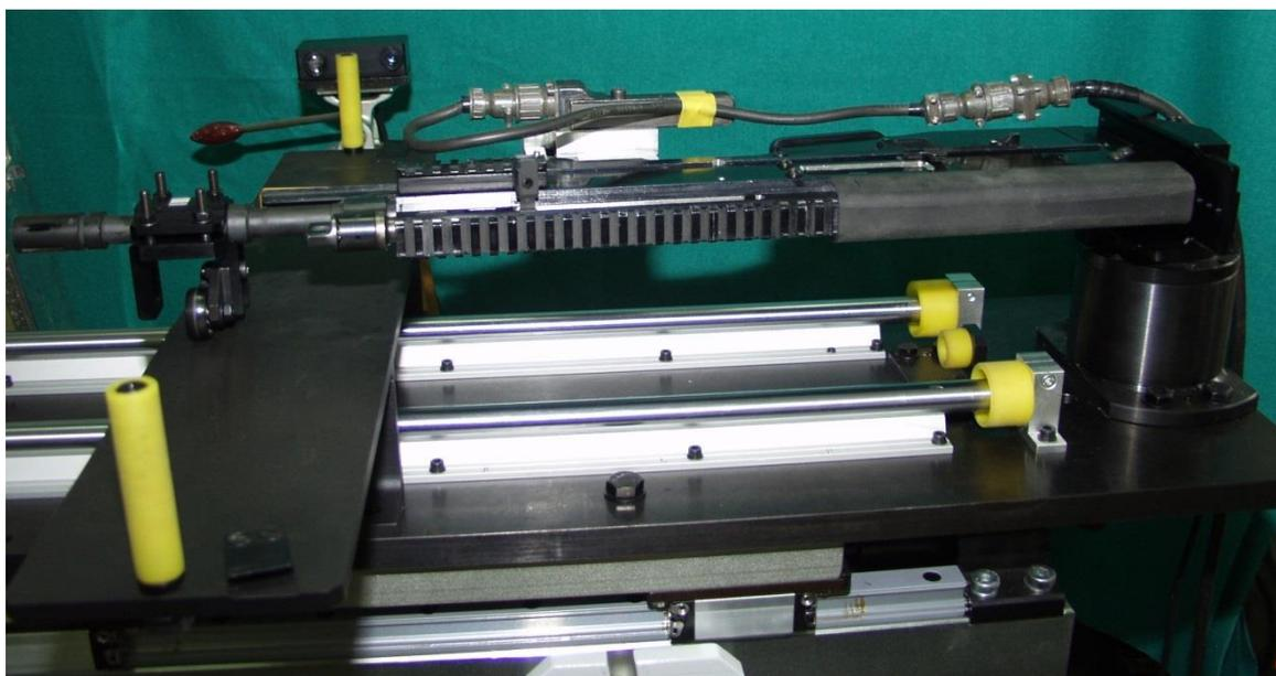
Fig. 13 MSBS-5,56 rifle during the weapon's jump angle measurement.
