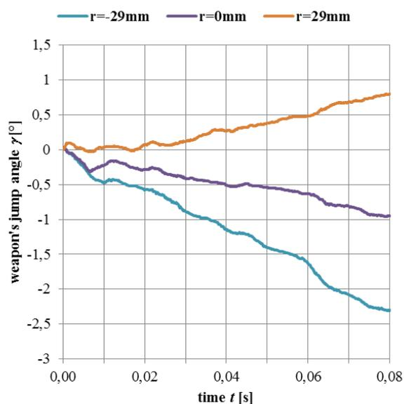
Fig. 14 MSBS-5,56 K-01 rifle experimental weapon's jump angle  $\gamma$  versus time  $t$ .
