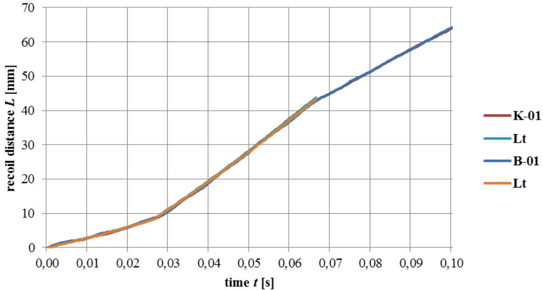
Fig. 16 Comparison of the Recoil distance  $L$  versus time  $t$  gained by the simulation and experiment.  $L_t$  – theoretical graphs
