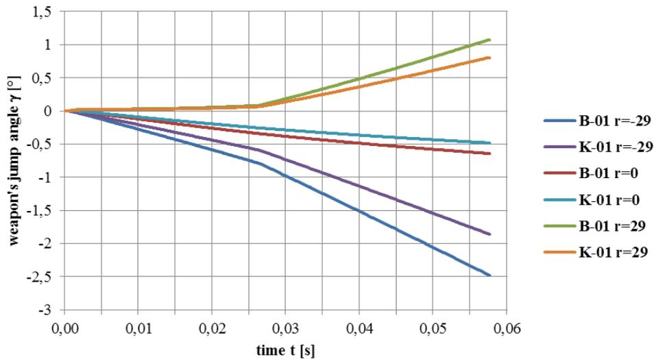
Fig. 8 Simulated weapon's jump angle  $\gamma$  versus time  $t$ .
