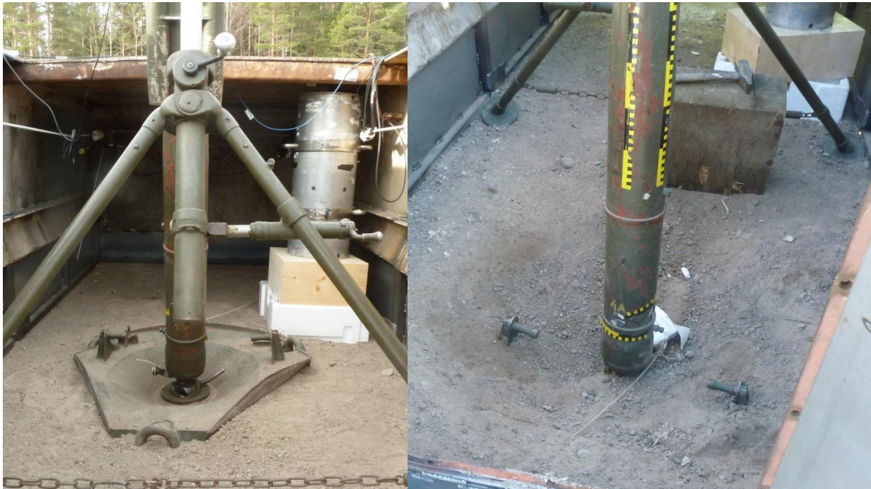
Figure 39 Baseplate pressed down in the ground by the recoil force
