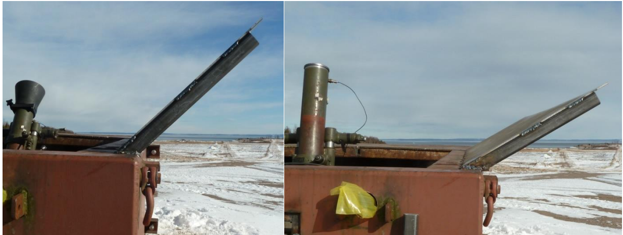
Figure 20. Different angle of the roof hatches (left: 45°, right: 30°)
