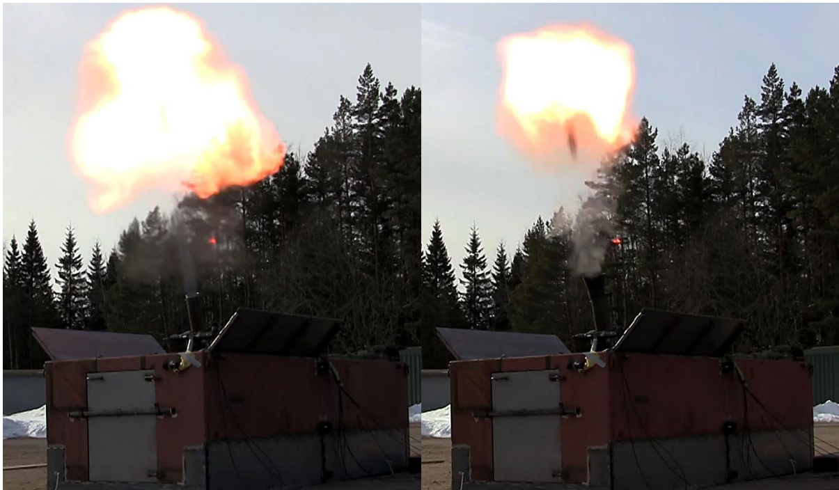
Figure 42 Difference in fire bolt; Left; without BAD, Right; with BAD
