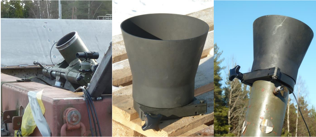
Figure 22. Left: Alteration of the barrel to fit the BAD. Middle: BAD. Right: BAD-mounted on the barrel
