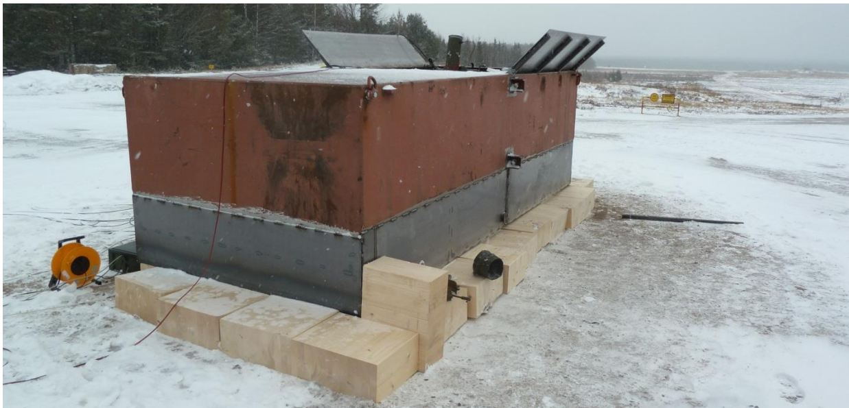
Figure 21. Elevation of the chassis with wooden blocks
