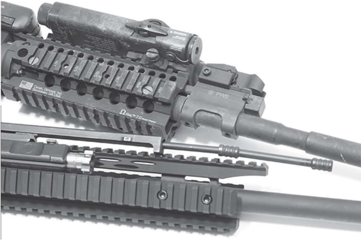
PWS makes a long-stroke piston system. Top is an early conversion, bottom is their dedicated piston system on one of their uppers.
