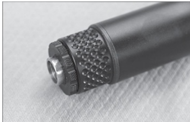
A Nielsen device, or L.I.D., that allows self-loading pistols to work with suppressors attached.
