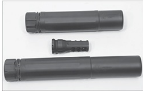
The Dead Air Armament S compared to the L, with a muzzle brake/mount in-between them.
