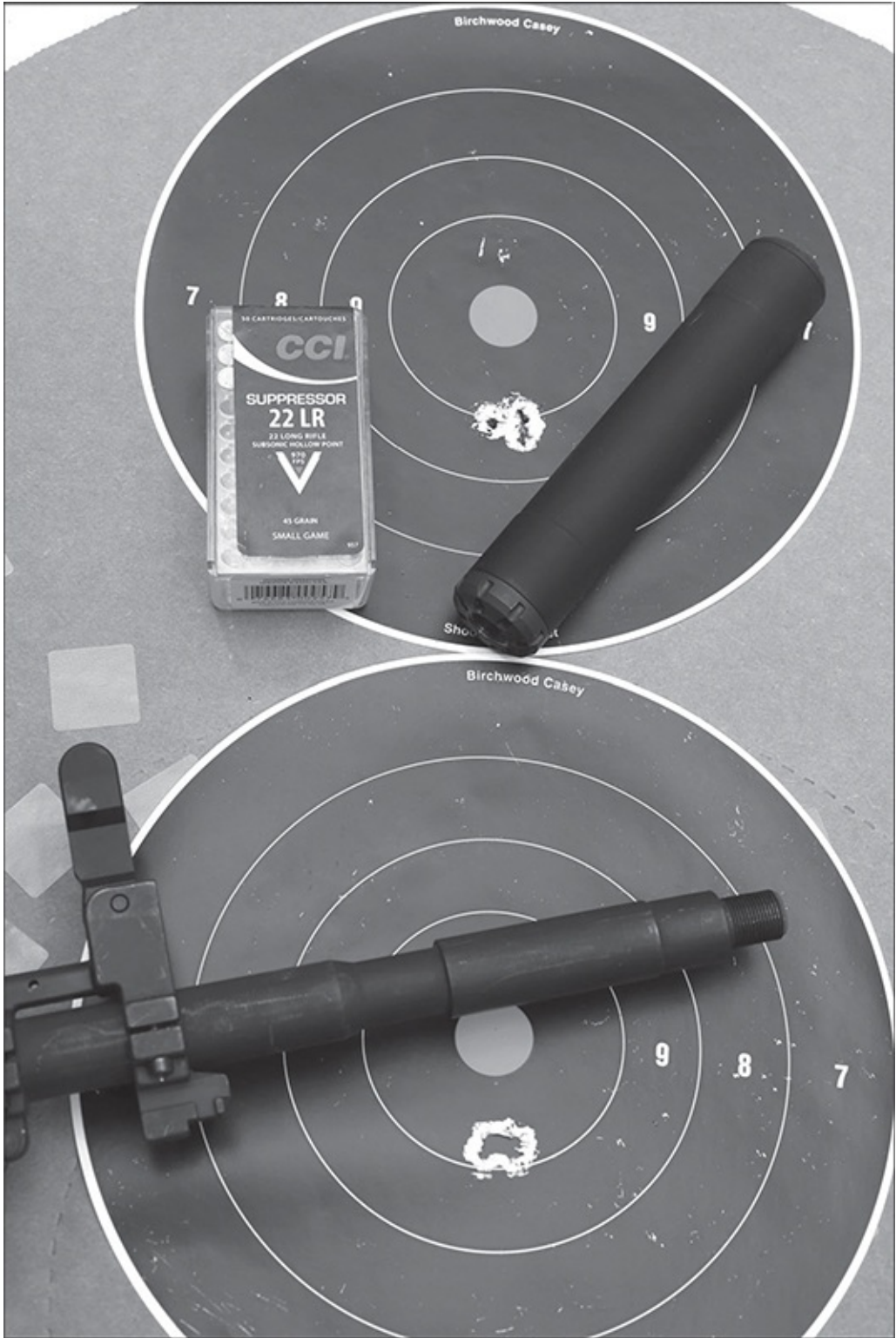
CCI 22LR ammo, CMMG rimfire conversion, and a Leupold scope. Groups with and without the Apex suppressor.
