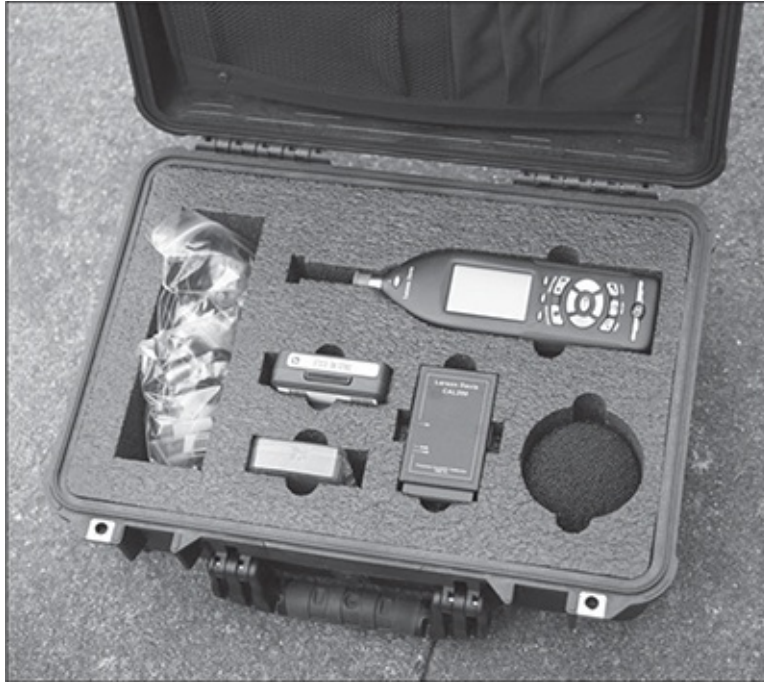
The complete kit, meter, microphone, instructions, calibration, hard case for storage and transport.
