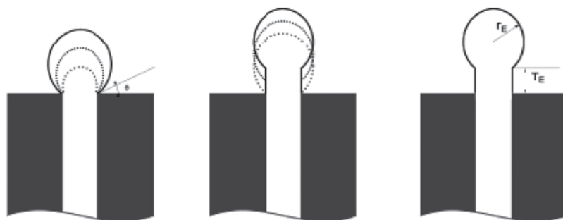
Fig. 1 Stagiile de formare a bulelor de gaze (Ramakrishnan et al. 1969; Satyanarayan et al. 1969)/
