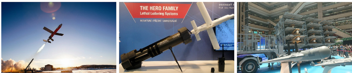
Fig. 1. Three examples of common launch methods for loitering munitions. Left: Fire shadow loitering munition launched by rail (image by Think Defence), middle: Hero-30 loitering munition which uses a canister launch method (image by Reise Reise), right: mobile launcher of multiple Chien hsiang loitering munitions (image by Kenchen 945).
