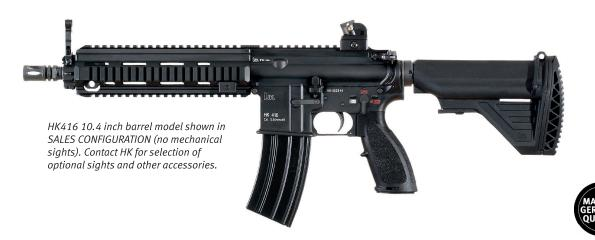
The HK416 is a 5.56x45mm magazine fed lightweight auto rifle available in multiple barrel lengths that is gas operated via short stroke gas piston system for enhanced reliability built on the common M4/M16/AR15 style platform. Often discussed as the multi-role weapon.
