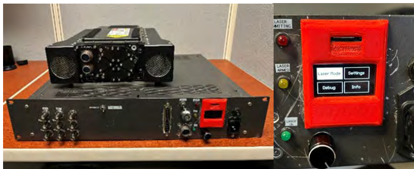
Figure 3. 2CIR missile warning simulator hardware and primary beam improvement
