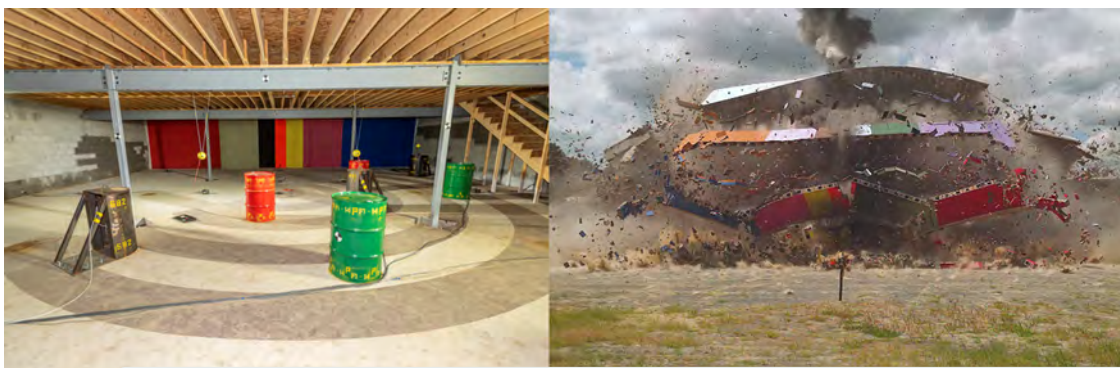
Figure 4. Two-story over-burial building debris test conducted in partnership with the U.S. Army Aberdeen Test Center at Aberdeen Proving Ground, Maryland
